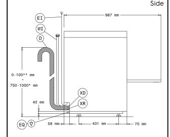
ΕI Electrical inlet (power) EO **Electrical Outlet** HWI Hot water inlet Rinse aid connection
